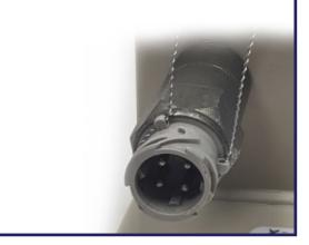
Pass the end of the wire through the remain free hole of the seal, so that on the other side may emerge +/- 4 cms.
