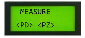
2. **<PD>** - read data from the sensor and then measure the current consumption.
