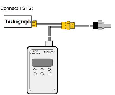
Make a test **<PZ>** on a moving vehicle. If the sensor works correctly, after some time, tachograph will display error (of cable, etc.).
