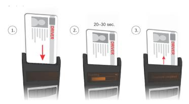
In order to make a driver card download with the device you have to insert the driver card into the card slot of the device in the way shown in picture.
