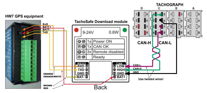
For a basic connection of a HW7 GPS unit follow the bellows schematic:
